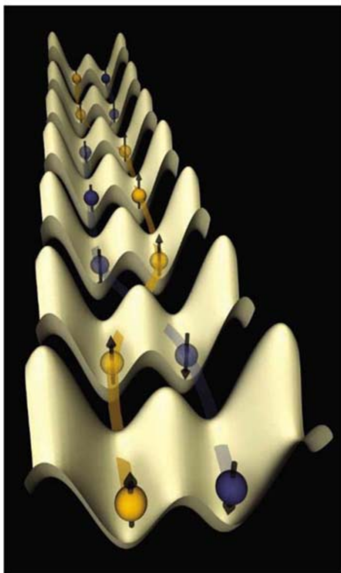
Atomic hopping. An array of double well potentials, where each well contains a single atom. Adjacent atoms interact through superexchange spin-spin coupling in which atoms quantum-mechanically tunnel from one well to the adjacent well and back, as studied by Trotzky et al.
